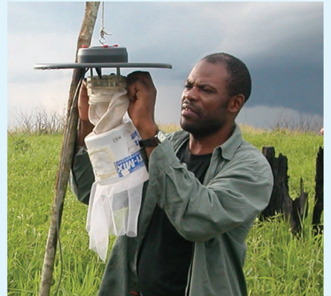
Kevin Njabo adjusting a CDC light trap. Baited with CO 2 , it is a tool to sample mosquitos for monitoring and surveilling disease vectors and other entomological surveys.
